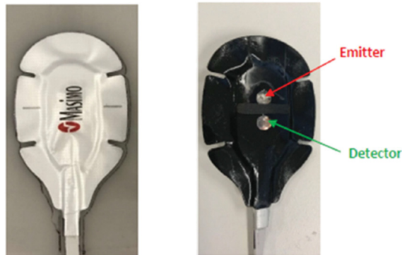
Single-detector device used in Dr. Madisetti's experiment. EX2001, Appendix p 1 (annotations in original)
