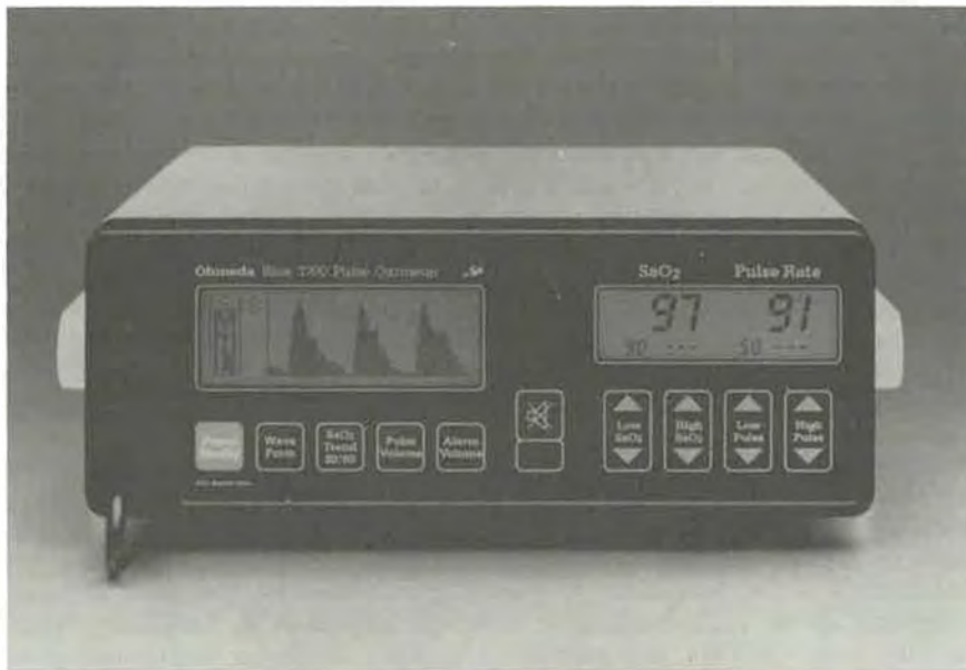
Figure 12.2 Front panel of Ohmeda Biox 3700 pulse oximeter (Courtesy of Ohmeda). The display at the left side shows real-time waveforms and pulse strength, while the display at the right side is used for alarm settings.
