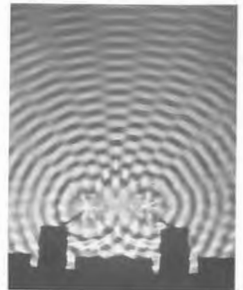
Figure 9.1 Water waves from two point sources in a ripple tank.
