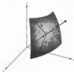
Figure 3.10 Portion of a spherical wavefront far from the source.
