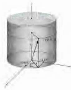
Figure 2.19 The geometry of cylindrical coordinates.
