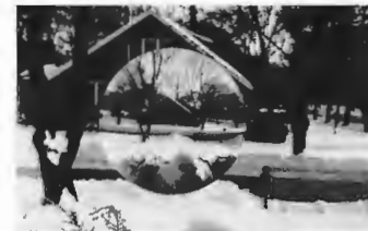
much as the eye projects its image on the retina. (d) The minified, rightside-up, virtual image formed by a negative lens.
