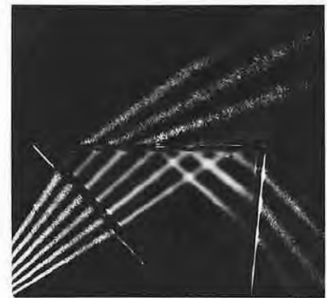
Figure 4.33 Internal reflection and the critical angle. (Photo courtesy of Educational Service, Inc.)
