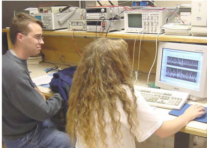
Figure 5. Two students acquire photoplethysmographic data in the AP 773 pulse oximetry laboratory (Fall 2002).
