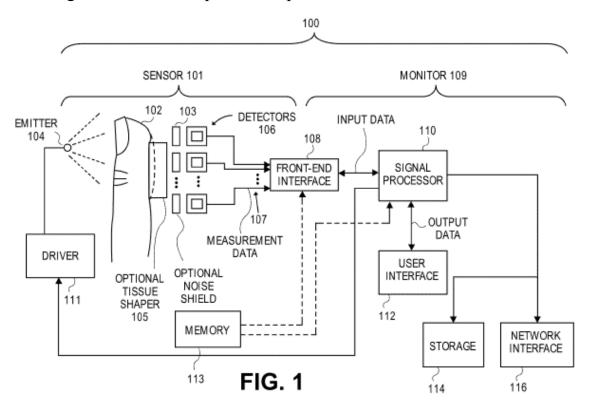
Figure 1 illustrates a block diagram of data collection system 100 including sensor 101 and monitor 109. *Id.* at 11:47–58. Sensor 101 includes optical
