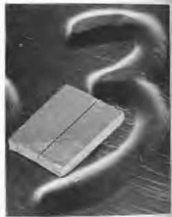
Figure 14.37 The cleaved-coupled-cavity laser. (Photograph by Bell Laboratories.)
