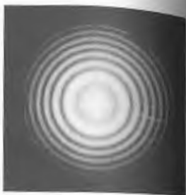
Figure 9.60 Fringes in scattered light.
