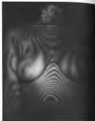
Figure 14.53 Double exposure holographic interferogram. (From S. M. Zivi and G. H. Humberstone, "Chest Motion Visualized by Holographic Interferometry," Medical Research Eng. p. 5 [June 1976].)
