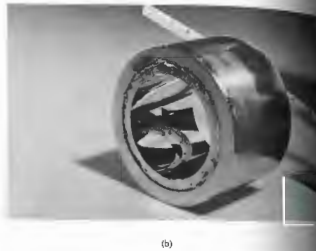
Figure 5.130 (a) X-ray focusing system. (b) X-ray mirror (Photo courtesy Lawrence Livermore National Laboratory.)
