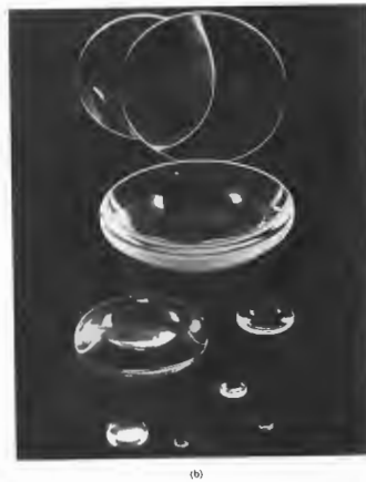
Figure 5.15 Cross sections of various centered spherical simple lenses. The surface on the left is #1 since it is encountered first. Its radius is R_1 . (Photo courtesy of Melles Griot.)
