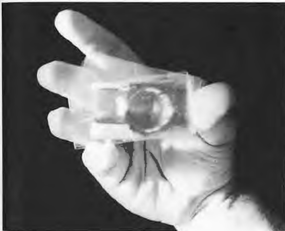
Figure 4.30 Near normal reflection off a stack of microscope slides. You can see the image of the camera that took the picture. (Photo by E.H.)
