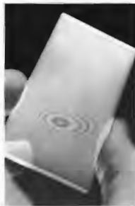
Newton's rings with two microscope slides. The thin film of air between the slides creates the interference pattern. (Photo by E. H.)
