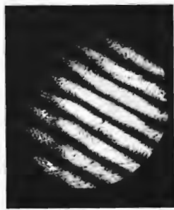
Interferogram without plasma. (Photo courtesy Los Alamos National Laboratory.)
