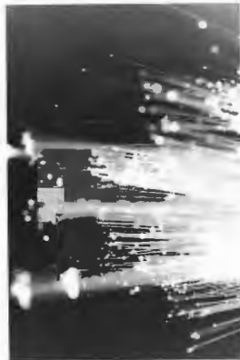
Light emerging from the ends of a loose bundle of glass fibers. (Photo by E.H.)
