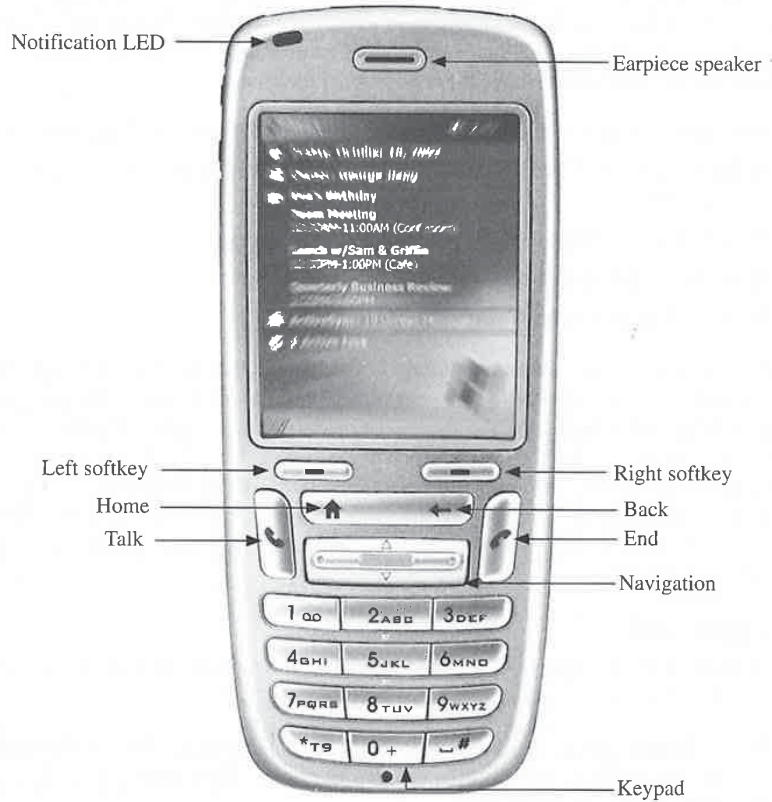
FIGURE 5-1 The front of a Smartphone (other Smartphones look different but have many of the same parts)
