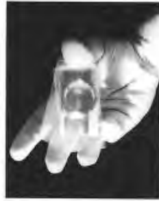
Near normal reflection off a stack of microscope slides. You can see the image of the camera that took the picture. (Photo by E.H.)
