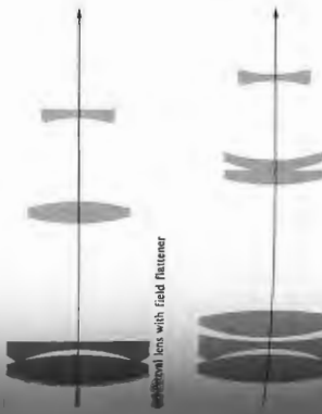
Figure 6.30 The field flattener.
