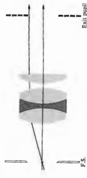
Figure 5.96 The orthoscopic eyepiece.
