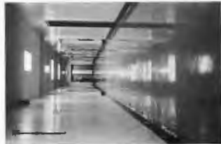
At near-glancing incidence the walls and floor are mirrorlike, despite the fact that the surfaces are rather poor reflectors at \theta = 0^\circ . (Photo by EKS)
