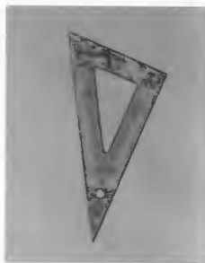
A clear plastic triangle between polaroids. (Photo by E. H.)
