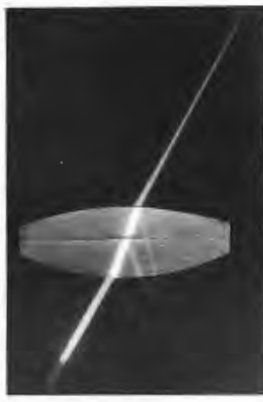
Figure 5.18 The focal plane of a lens.
