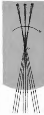
Figure 5.17 Focusing of several ray bundles.
