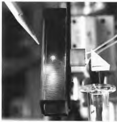
The tiny starlike speck is a minute (one-thousandth of an inch diameter) transparent glass sphere suspended in midair on an upward 250-mW laserbeam. (Photo courtesy Bell Laboratories.)
