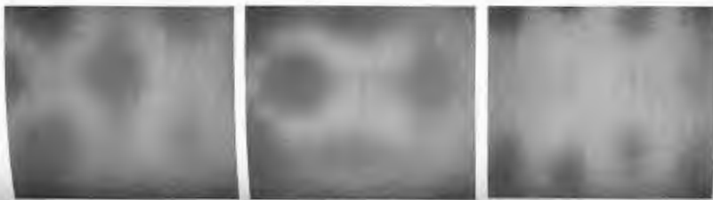
Three-dimensional electromagnetic standing-wave pattern. The heights inside a microwave oven. (Photo courtesy Atsuhiko Uchida, University of Tsukuba.)
