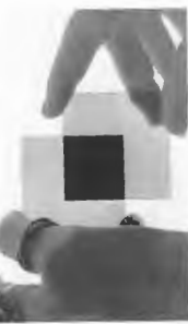
Figure 8.3 Dichroism 335 A pair of crossed polaroids. Each polaroid appears gray because it absorbs roughly half the incident light. (Photo by E.H.)
