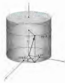
Figure 2.19 The geometry of cylindrical coordinates.
