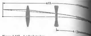
Figure 5.113 A telephoto lens.
