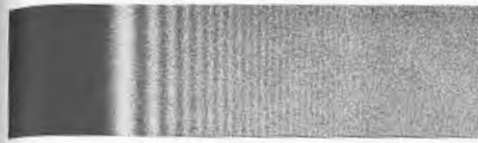
Figure 10.75 The fringe pattern for a half-screen.
