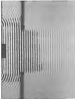
Figure 10.82 Ripple-tank waves passing through a slit. (Photo courtesy PSSC Physics, D. C. Heath, Boston, 1960.)
