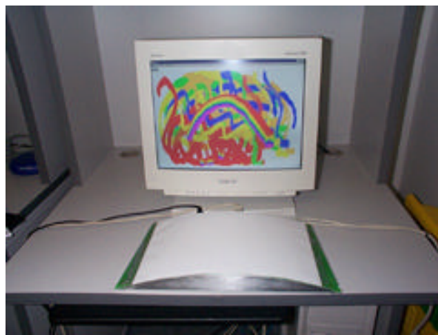
Figure 1: The Multi-Touch Surface and attached monitor. Finger strokes made on the board are transformed into paint strokes on the screen.
