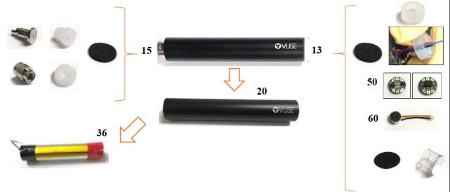
The PCBA drives the heater coil and two LEDs and is connected to the pressure sensor, the battery PCM and the battery electrode using solder. The pressure sensor is a commercial off-the-shelf (COTS) item that detects vacuum draw on the device relative to ambient pressure, which gains access to the pressure sensor by two thru holes in the PCBA.
