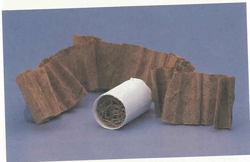
PLATE 2.13.2-1 Photograph of the assembled tobacco-paper filter (foreground) and the tobacco-paper used to construct it.
