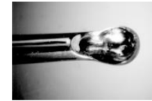
Figure 1 The tip of the 'gonioscraper'. The bowl is 300 µm in diameter with its edges sharpened.
