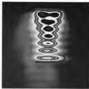
A two-dimensional standing wave pattern formed between a source and a reflector. EM waves from a 3.0-GHz antenna enter from the right. They reflect off a metal rod and travel back to the antenna. The pattern is made visible by absorbing the microwave radiation and recording the resulting temperature distribution with an R Camera. (Photo courtesy R. H. Pohl, Philips Laboratory, Eindhoven, The Netherlands.)
