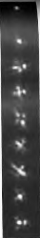
When looking through the atmosphere with a telescope the probability of experiencing a moment of clear viewing decreases exponentially with aperture diameter. Using a moderate-size objective (=12-inch) in ordinary seeing conditions the odds are 1 in 100. This sequence of photos of a star taken at 1/200-second intervals shows how the image "winkles." The right-most picture was taken at an instant of very good seeing. With diffraction-limited instrument the image should resemble the Airy disk pattern (p. 479) of a central bright spot surrounded by faint concentric rings. (Photo courtesy Ron Daniwicz, Museum of Science, Boston.)
