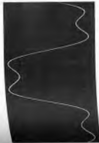
Figure 7.29 Synthesis of the profile of a periodic square wave. Notice that the constituent waves are in phase and zero whenever the square wave is zero. Since all the sine waves are in phase at x = 0 , all the coefficients are positive. (Made by E. H.)
