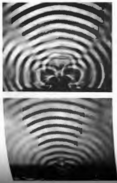
Figure 10.1 In one case, the waves are simply diffracted by a slit; in the other, a series of equally spaced point sources span the aperture and generate a similar pattern. (Photos courtesy PSSC Physics, D. C. Beeson, 1960.)
