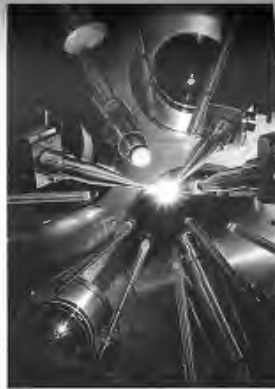
Inside the target chamber of the LLE laser-fusion device. Fusion reactions take place in a tiny target sphere filled with deuterium/tritium, 30 \mu\text{m} in diameter, which is irradiated by the 30-kJ Omega laser. (Photo courtesy University of Rochester Laboratory for Laser Energetics; Eugene Kowalski, Image Specialist.)
