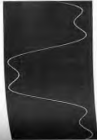
Figure 7.29 Synthesis of the profile of a periodic square wave. Notice that the constituent waves are in phase and zero wherever the square wave is zero. Since all the sine waves are in phase at x = 0 , all the coefficients are positive. (Made by E. H.)
