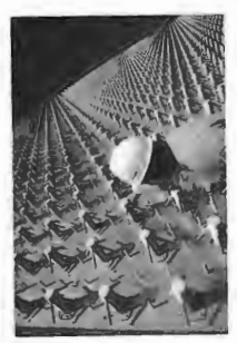
A modern phased-array radar system. The field of individual small antennas behaves very much like the atoms on a smooth surface. By introducing a proper phase shift between adjacent rows the antenna can "look" in any direction. A reflecting surface has a similar phase shift determined by \theta as the incident wave sweeps over the array of atoms. (Courtesy Raytheon Corp.)
