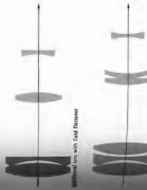
Figure 6.30 The field flattener.
