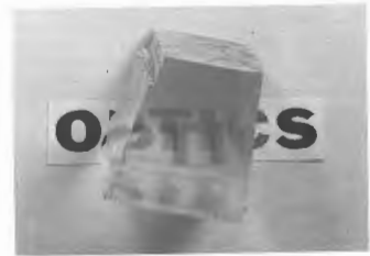
Figure 8.20 Double image formed by a calcite crystal (not cleavage form). (Photo by Z.H.)
