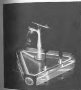
A ring laser gyro. (Photo courtesy Autonetics, a Division of Rockwell Corp.)
