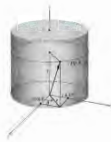
Figure 2.19 The geometry of cylindrical coordinates.
