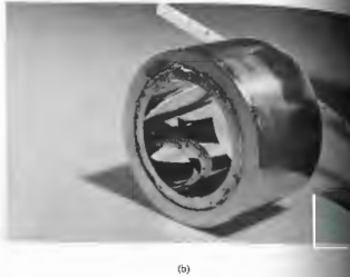
Figure 5.130 (a) X-ray focusing system. (b) X-ray mirrors (Photo courtesy Lawrence Livermore National Laboratory.)
