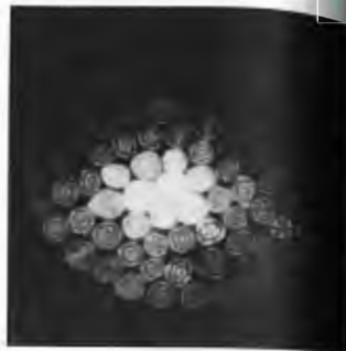
Figure 5.68 Optical waveguide mode patterns seen in the end view of small-diameter fibers. (Photo courtesy of Narinder S. Ghosh.)
