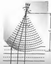
Figure 5.9 The reshaping of plane into spherical waves at a spherical interface— F_i is the image focus.
