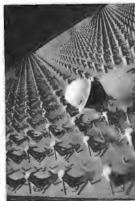
A modern phased-array radar system. The field of individual small antennas behaves very much like the atoms on a smooth surface. By introducing a proper phase shift between adjacent rows the antenna can "look" in any direction. A reflecting surface has a similar phase shift determined by \theta as the incident wave sweeps over the array of atoms. (Courtesy Raytheon Corp.)
