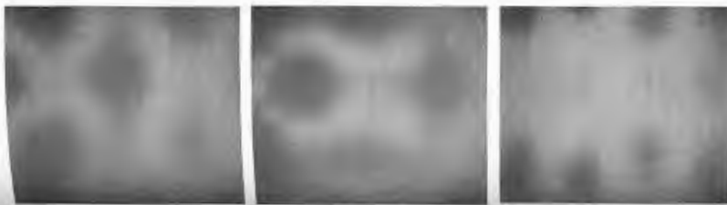
Three-dimensional electromagnetic standing-wave pattern. The heights inside a microwave oven. (Photo courtesy Atsuhiko Uchida, University of Hawaii.)
