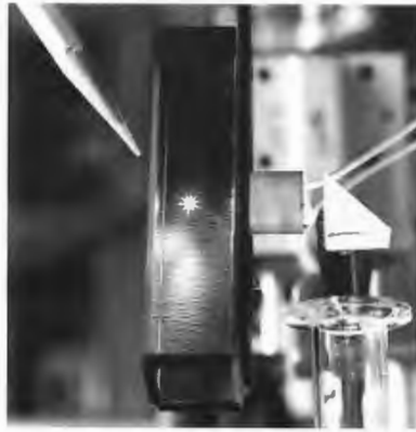
The tiny starlike speck is a minute (one-thousandth of an inch diameter) transparent glass sphere suspended in midair on an upward 250-mW laserbeam. (Photo courtesy SRI Laboratories.)
