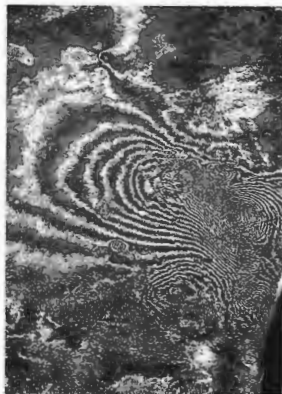
Synthetic aperture radar was used to produce this interferogram arising from the June 1992 earthquake in Landers, California. Images taken by the ERS-1 satellite before and after the quake were combined to generate this fringe pattern which reveals the shift in the ground that took place. The picture covers an area of about 125 by 175 km. (Photo courtesy Didier Meunier, Centre National d'Etudes Spatiales, France.)
