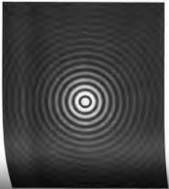
Bessel beam. (Photo courtesy Ryan P. McDonald.)
