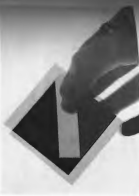
A hand holding a piece of Scotch tape stuck to a microscope slide between two crossed polaroids. (Photo by E.H.)
