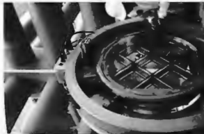
The KDP frequency converter for the Nova laser. (Photo courtesy Lawrence Livermore National Laboratory.)
