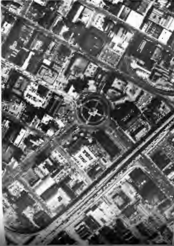
(a) New Orleans and the Mississippi River photographed from 12,500 m (41,000 ft) with Itek's Methrac-21 camera ( f = 21 cm). Ground resolution, 1 m; scale, 1:59,492. (b) Photo scale, 1:10,000. (c) Photo scale, 1:2500. (Photos courtesy of Litovitz Optical Systems.)
