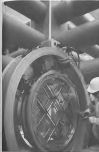
Figure 14.59 The KDP frequency converter for the Nova laser. (Photo courtesy Lawrence Livermore National Laboratory.)
