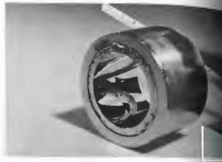
Figure 5.130 (a) X-ray focusing system. (b) X-ray mirrors (Photo courtesy Lawrence Livermore National Laboratory.)
