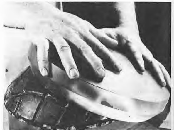
Figure 5.7 Polishing a spherical lens. (Photo courtesy Optical Society of America.)
