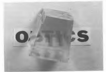
Figure 8.20 Double image formed by a calcite crystal (not cleavage form). (Photo by Z.H.)
