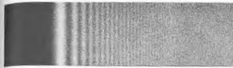
Figure 10.75 The fringe pattern for a half-screen.
