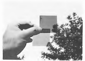
Figure 8.38 A pair of crossed polarizers. The upper polaroid is noticeably darker than the lower one, indicating the partial polarization of sky light. (Photo by E.H.)
