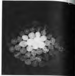
Figure 5.68 Optical waveguide mode patterns seen in the end views of small-diameter fibers. (Photo courtesy of Narinder S. Ghosh.)
