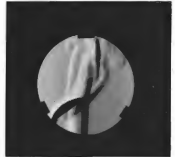
Figure 14.22 A schlieren photo of a spoon in a candle flame. (Photo by E. H.)
