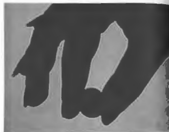
Figure 10.1 The shadow of a hand holding a dime, cast directly on 4 × 5 Polaroid A.S.A. 3000 film using a He-Ne beam and no lenses. (Photo by E.H.)
