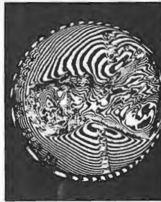
Interferometric image of a penny via acoustical holography. (Photo courtesy HoloScience, Inc.)
