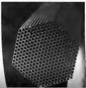
Figure 5.78 A scanning electron micrograph of a single multichannel thread containing bundles of hollow capillaries. (Photo courtesy Atay Optical Systems, Inc.)
