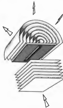
Figure 2.28 Cylindrical waves emerging from a long, narrow slit.
