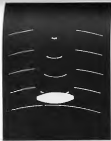
The actual wavefronts of a diverging lightwave partially focused by a lens. The photo shows five exposures, each separated by about 10 ns (i.e., 100 \times 10^{-12} s), of a spherical pulse 10 ps long as it sweeps through a converging lens. The picture was made by using a photographic technique. (Courtesy of N.H. Abramson.)
