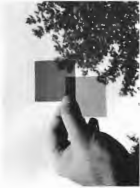
A pair of crossed polarizers. The upper polaroid is noticeably darker than the lower one, indicating the partial polarization of sky light. (Photo by E.H.)
