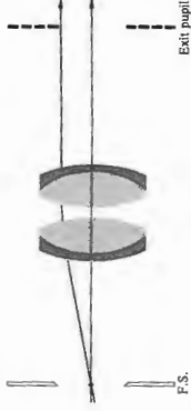
Figure 5.97 The symmetrical (Plossl) eyepiece.
