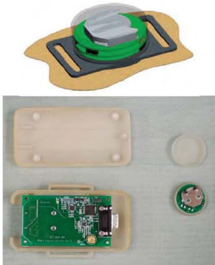
Fig. 1. (Top) Attachment of Sensor Module to the skin; (Bottom) photograph of the Receiver Module (left) and Sensor Module (right).
