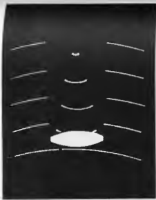
The actual wavefronts of a diverging lightwave partially focused by a lens. The photo shows five exposures, each separated by about 10 ps (i.e., 100 \times 10^{-12} s), of a spherical pulse 10 ps long as it sweeps through a converging lens. The picture was made by using a photographic technique. (Courtesy of N.H. Abramson.)
