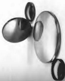
A number of semiconductor lenses made from ZnSe, CdTe, GaAs, and Si. These materials are particularly useful in the infrared ( 2 \mu\text{m} to 30 \mu\text{m} ). They are highly transparent despite the fact that they are opaque in the visible region of the spectrum. (Photo courtesy, Hewlett-Packard.)
