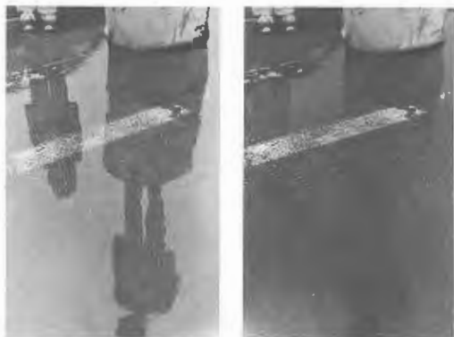
Figure 8.41 Light reflected off a puddle is partially polarized. (a) When viewed through a Polaroid filter whose transmission axis is parallel to the plane of incidence, most of the glare is visible. (b) When the filter's transmission axis is perpendicular to the plane of incidence, most of the glare is removed. (Photo courtesy: Mark Seymour.)
