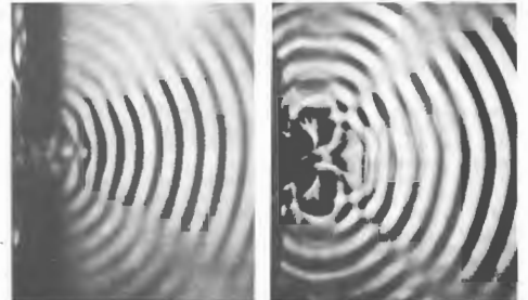
Figure 10.4 Ripple-tank photos. In one case the waves are simply diffracted by a slit; in the other, a series of equally spaced point sources span the aperture and generate a similar pattern. (Photos courtesy PSSC Physics, D. C. Heath, Boston, 1960.)
