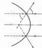
Figure 5.45 Real and virtual images for a paraboloidal mirror.
