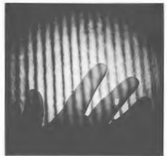
Figure 9.36 Real Michelson fringes using He-Ne laser light. (Photo by E. H.)
