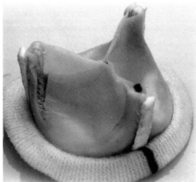
Fig. 7. Failed ISU valve from the fatigue tests
