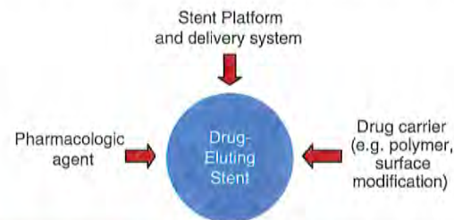
Figure 31.4 Components of drug-eluting stents.
