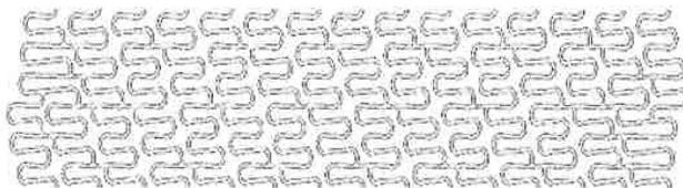
Figure 13.1: Structure of the GENIC coronary stent.
