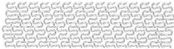
Figure 13.1: Structure of the GENIC coronary stent.
