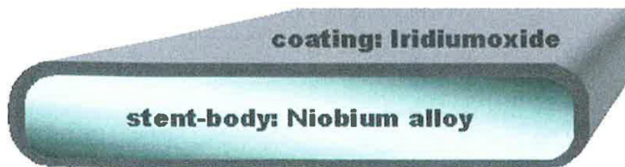
Figure 17.4: Schematic cross-sectional drawing highlighting the special construction of the Lunar stent. The Niobium core of the stent is covered with the iridium oxide. The Niobium alloy is a heavy-metal-free material, with the same mechanical features as steel. This corrosion-free clinically proven material has self-healing features. The iridium oxide decreases the formation of free oxygen radicals, and thus decreases the inflammatory stimulus after stent implantation.
