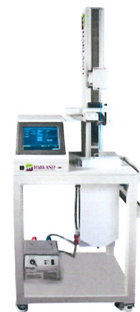
A friction test system to measure lubricity.
