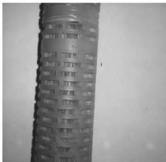
Figure 7 Oxidative coloration and disintegration of an air filter. Source: Courtesy of Sartorius Stedim GmbH.
