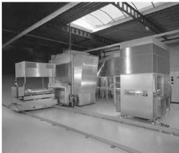
Figure 11 Lyophilizer transfer cart with loader and unloader (13).
