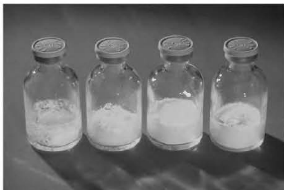
Figure 7 The vial on the left shows complete collapse and the second vial from the left is an example of partial collapse. The two vials on the right are pharmaceutically acceptable.
