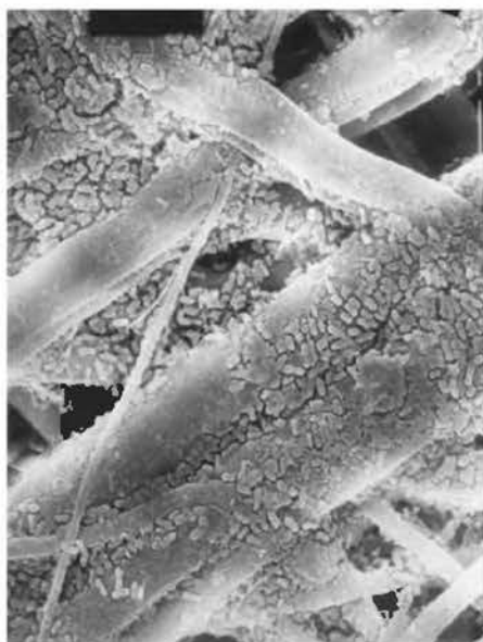
Figure 6 Microorganisms captured on glass fiber. Source: Courtesy of Sartorius Stedim GmbH.
