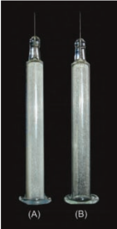
Figure 4: Comparison of siliconisation methods. Sewa's in-house method used on syringe (A) and standard spray method used on syringe (B).
