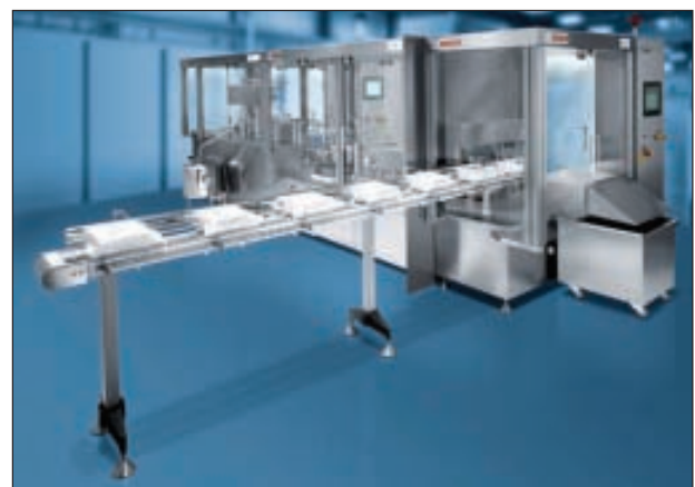
Figure 3: Two views of a high performance syringe line with fully automatic bag opening (ABO), fully automatic tub opening (ATO) and filling machine FXS 5100 with integrated In-Process-Checkweigh.
