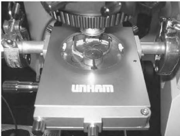
Figure 10 Stage for freeze dry microscopy.
