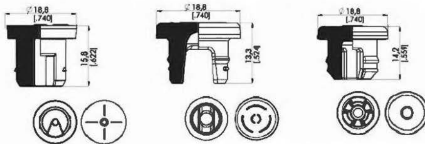
Figure 6 20 mm lyophilization stoppers in various product designs.
