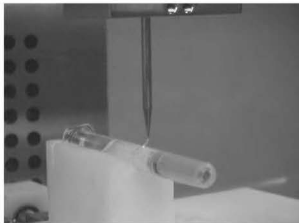
Figure 2 A glass prefilled syringe containing an aqueous liquid being tested using Nikka Densok's electrical conductivity method. Positive electrical current occurred near a laser drilled hole in the glass barrel wall. Source: Courtesy of Nikka Densok, Inc., Lakewood, Colorado, U.S.
